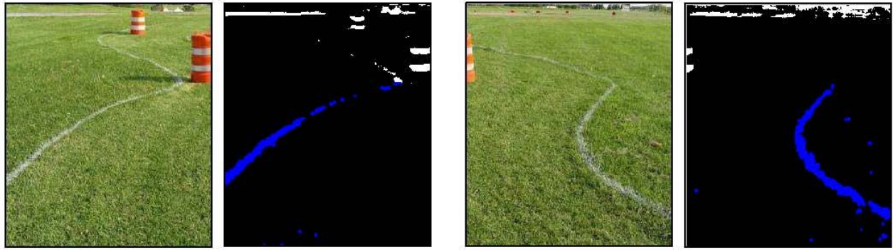
Figure 8: Line detection Left is the original image, Right is the image before transformed into binary image.
